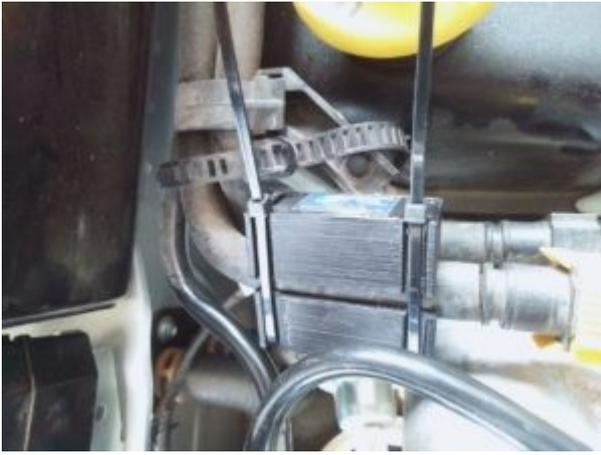
Place over the rubber or plastic fuel line and secure it with the plastic ties. Make sure the gap on either side of the fuel line is about the same. **DO NOT OVER TIGHTEN.**
