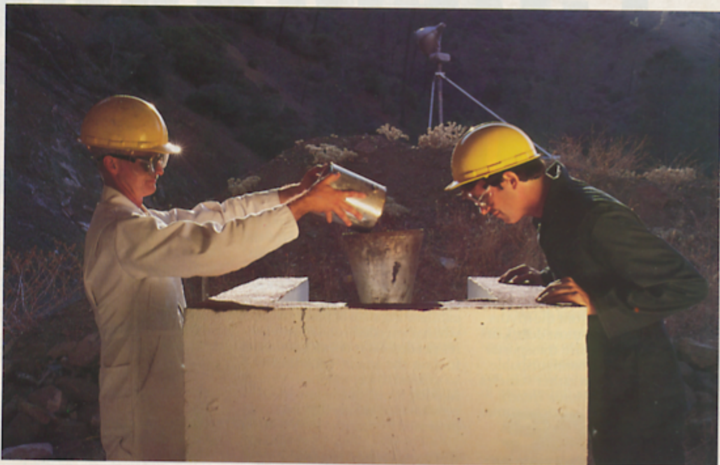
Al Kraft and Tom Pavia rehearse pouring propellant into a funnel to produce a rocket motor.
